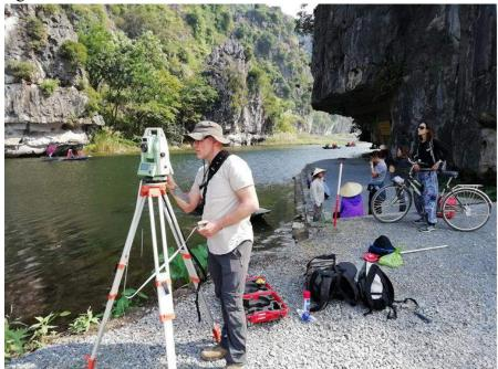
Figure 2. Notch survey at Thanh Warf, Thai Vy using a Leica TS06 total station (Source: E. Hill)
